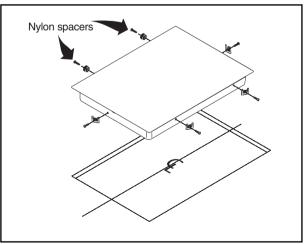
Install the retainer brackets to the bottom of the cooktop; then snug the bolts against the bottom of the countertop as shown.
